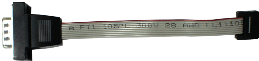
Figure 33: DE9 cable for the COM1 connector
