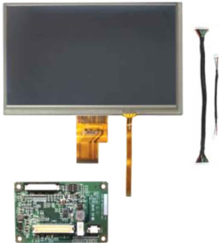
Figure 37: optional EDM Display kit (TDHJ070NA4RESKIT))
