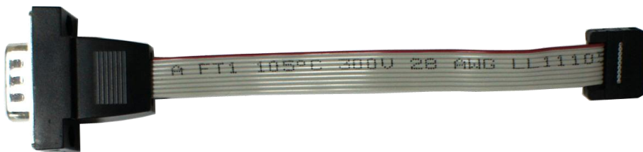
Figure 32: DE9 cable for the CAN BUS2 connector
