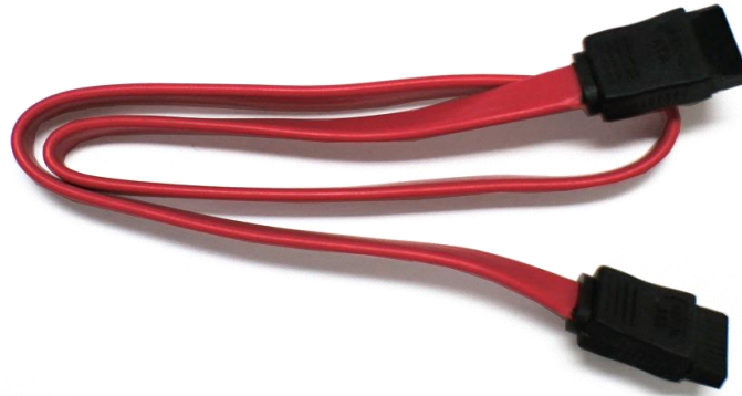
Figure 27: SATA DATA Cable for the SATA1 connector
