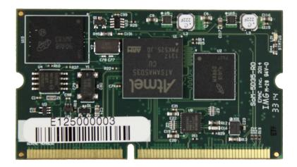
This document describes EMAC's SoM-A5D35 System on Module. The SoM-A5D35 is designed to be compatible with EMAC's 144-pin SODIMM form factor. This module is built around the ATMEL AT91SAMA5D35 microcontroller, which provides several of its key features.
