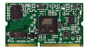
This document describes EMAC's SoM-9X25M (SBC) module. The SoM-9X25M is a System on Module, designed to be compatible with EMAC's 144-pin SODIMM form factor. This module is built around the ATMEL AT91SAM9X25 microcontroller, which provides several of its key features.
