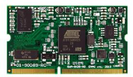
This document describes EMAC's SoM-9X25M (SBC) module. The SoM-9X25M is a System on Module, designed to be compatible with EMAC's 144-pin SODIMM form factor. This module is built around the ATMEL AT91SAM9X25 microcontroller, which provides several of its key features.
