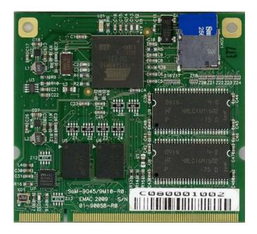
This document describes EMAC's SoM-9G45M & SoM-9M10M System on Modules (SoMs). The SoM-9G45/9M10 is a System on Module, designed to be compatible with EMAC's 200-pin SODIMM form factor. This module is built around the Atmel AT91SAM9G45 & AT91SAM9M10 ARM based microcontrollers, which provide several of its key features. Revision 2.x of this manual references SoM-9G45 / 9M10 PCB Revision 2 or better. See SoM-9G45 / 9M10 Revision 2.0 Product Change Notification for details.
