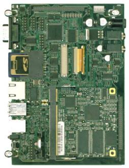
If using the SoM-9M10's external bus, it is highly recommend to buffer the bus on the carrier board in close proximity to the SoM SODIMM connector (see the SoM-200 carrier schematics for reference).
