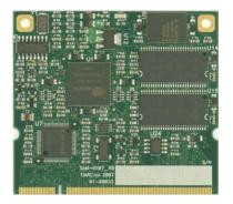
This document describes EMAC's SoM-9307M (SBC) module. The SoM-9307M is a System on Module, designed to be compatible with EMAC's 200-pin SODIMM form factor. This module is built around the Cirrus EP9307 microcontroller, which provides several of its key features.
