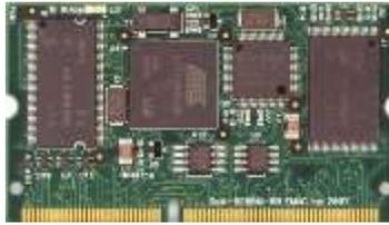
This document describes EMAC's SoM-9260M (SBC) module. The SoM-9260M is a System on Module, designed to be compatible with EMAC's 144-pin SODIMM form factor. This module is built around the ATMEL AT91SAM9260 microcontroller, which provides several of its key features.
