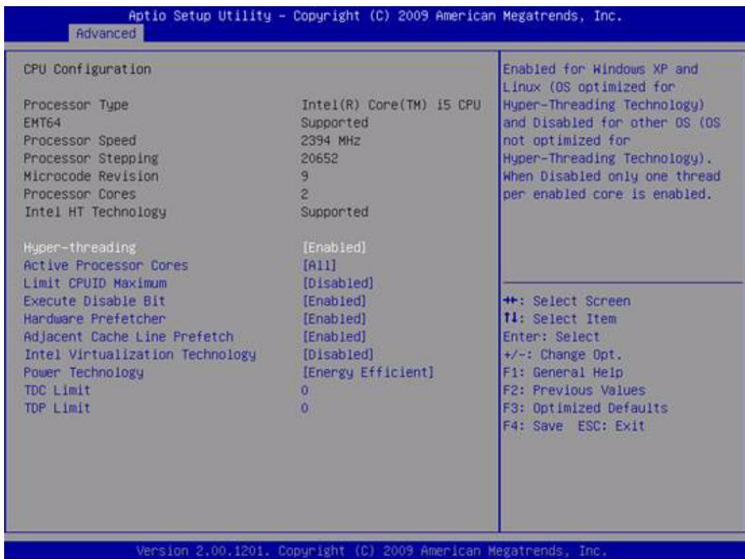
Figure 3.6 CPU Configuration
