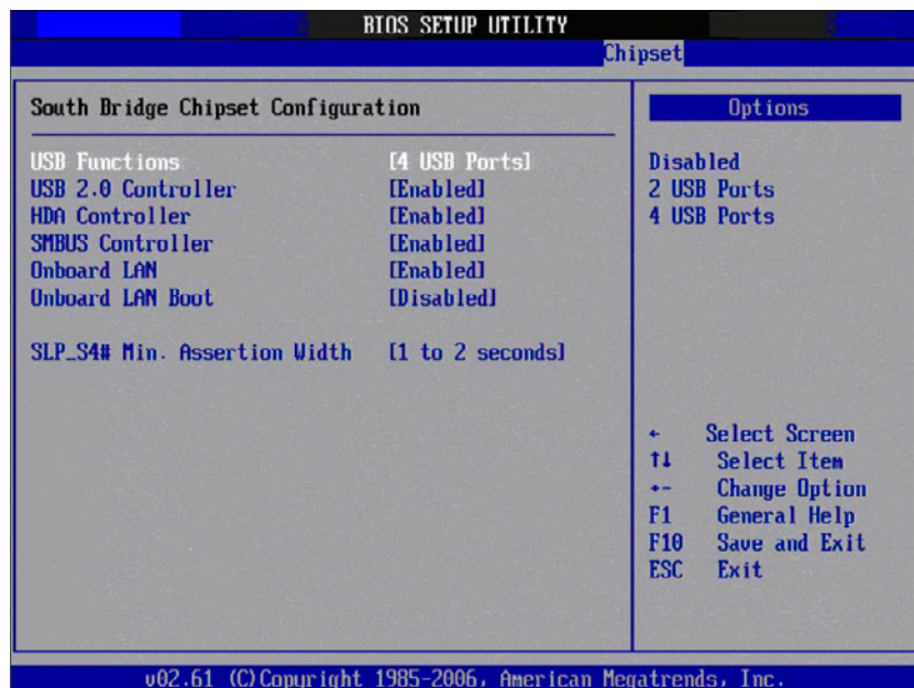
Figure 3.27 South Bridge Configuration
