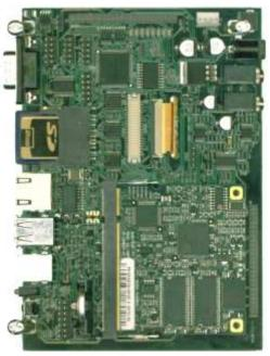
If using the SoM-3517's external bus, it is highly recommended buffering the bus on the carrier board in close proximity to the SoM SODIMM connector, (see the SoM-200 carrier schematics for reference).
