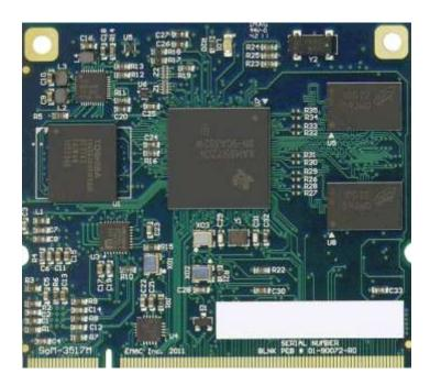
This document describes the EMAC SoM-3517M System on Module. The SoM-3517M is designed to be compatible with EMAC's 200-pin SODIMM form factor. This module is built around the Texas Instruments AM3517 ARM Cortex A8 based microprocessor, which provides several of its key features.
