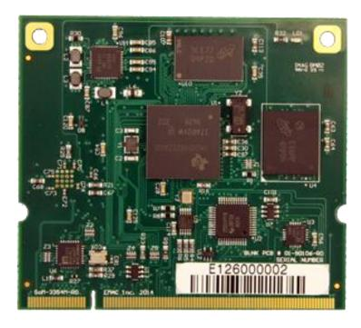
This document describes the EMAC SoM-3354M System on Module. The SoM-3354M is designed to be compatible with EMAC's 200-pin SODIMM form factor. This module is built around the Texas Instruments AM3354 ARM Cortex-A8 based microprocessor, which provides several of its key features.
