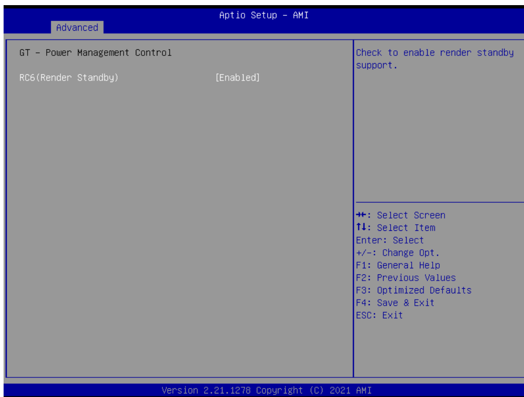
Figure 3.11 GT- Power Management Control
