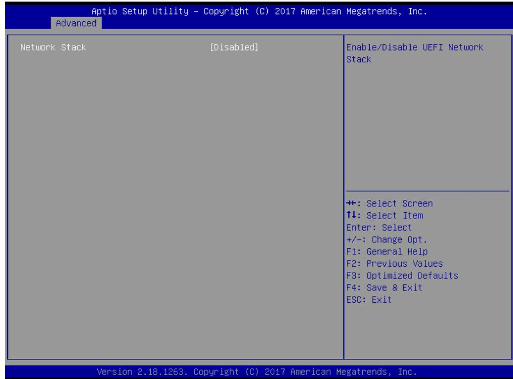
**Figure 3.29 Network Stack Configuration**
