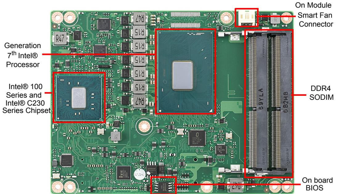
Figure 2.1 Board chips identify – Front
