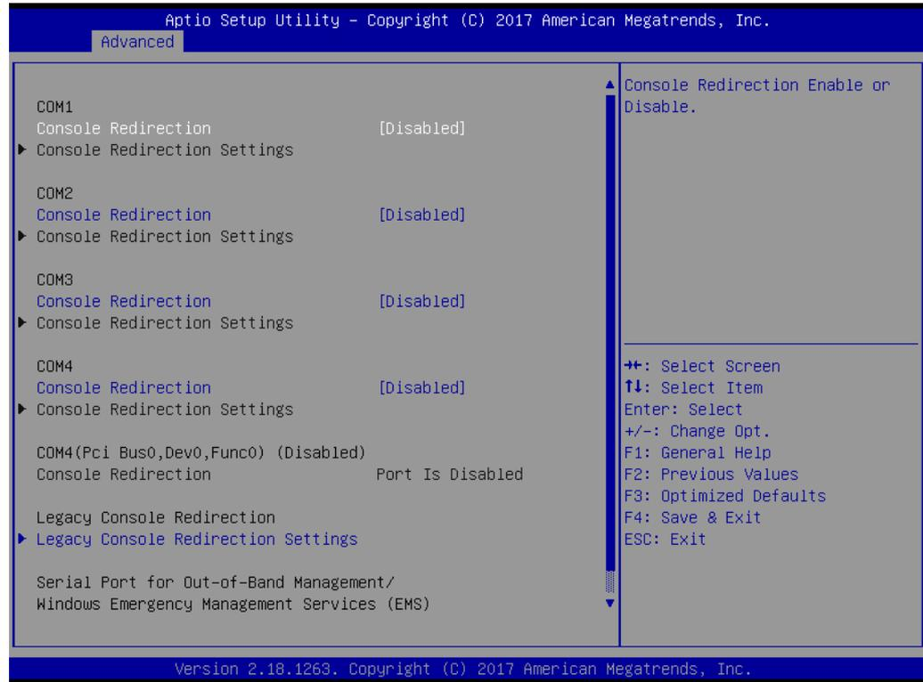
**Figure 3.27 Serial Port Console Redirection**
