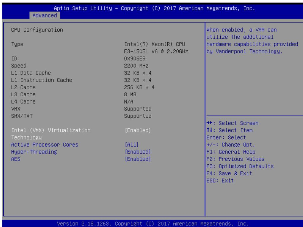
**Figure 3.4 CPU Configuration**
