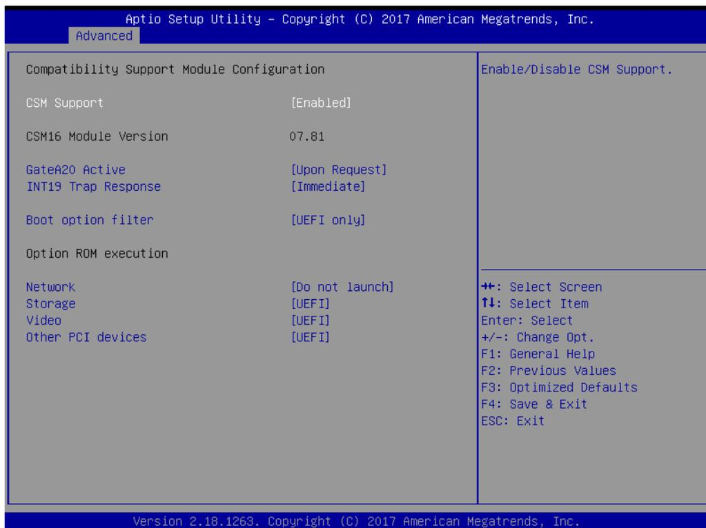
**Figure 3.30 CSM Configuration**
