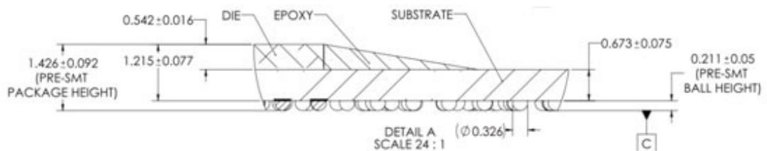
**Figure 2.8 PCH Height and Tolerance**
