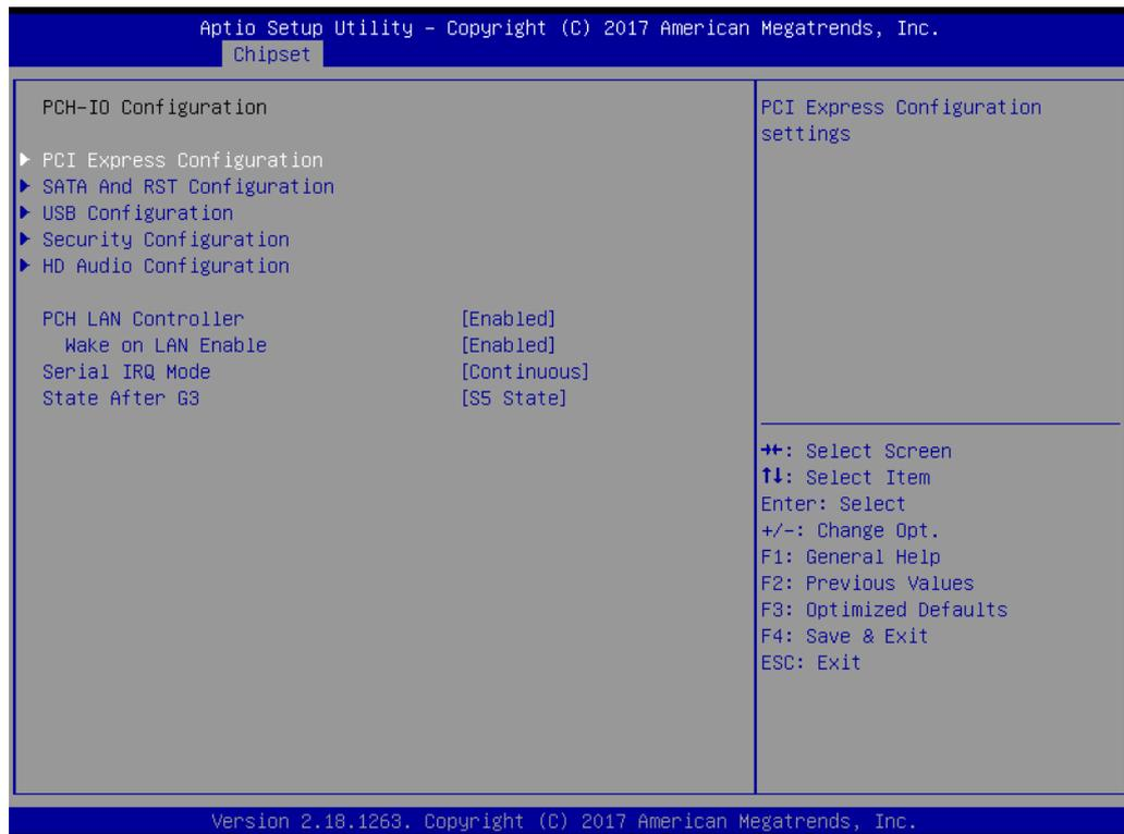
Figure 3.41 PCH-IO Configuration
