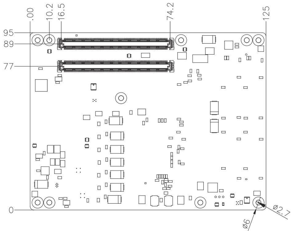
**Figure 2.4 Board Mechanical Drawing – Rear**
