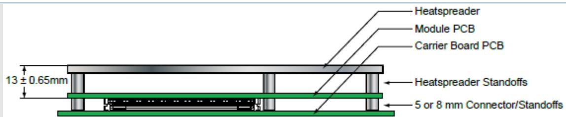
Cooling solutions provided from Kontron Europe GmbH for basic sized Computer-on-Modules are 27mm in height from module bottom to Heatsink top.
