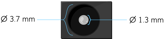
Figure 5: DC-In jack diagram
