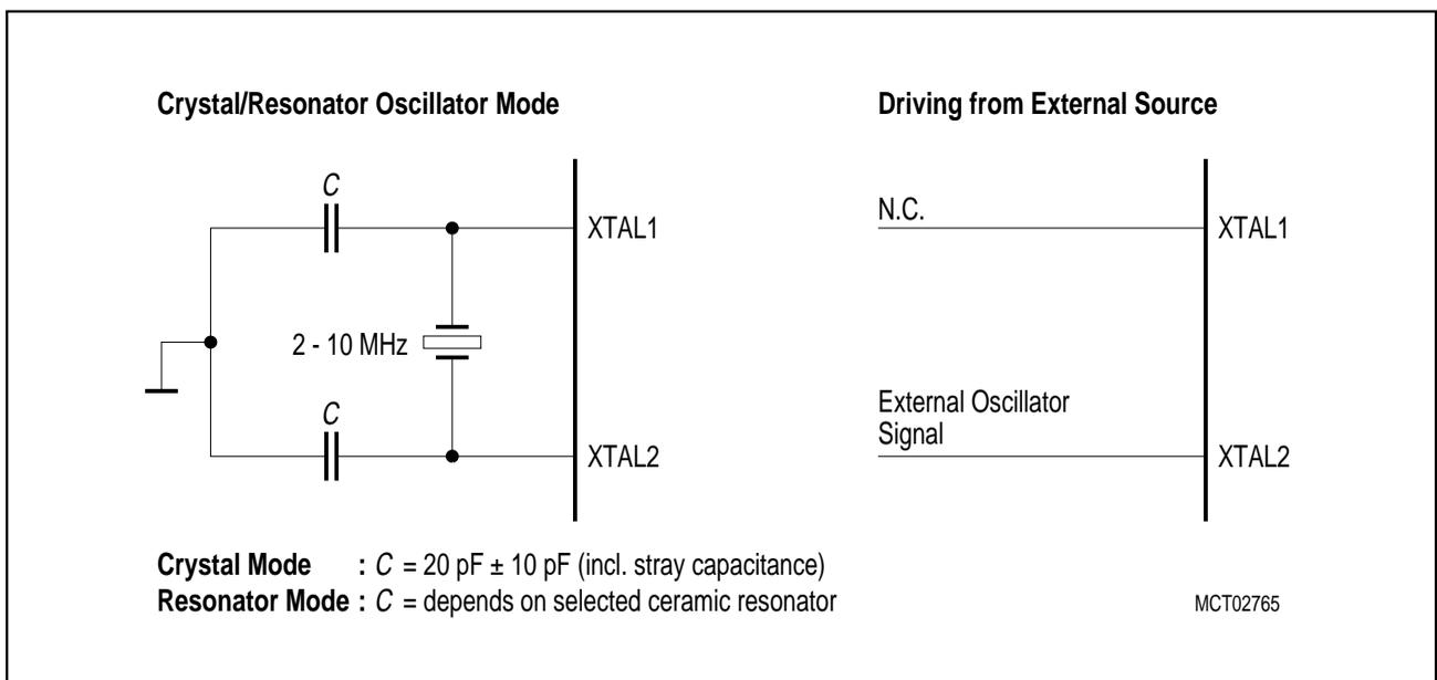
**Recommended Oscillator Circuits for Crystal Oscillator**
