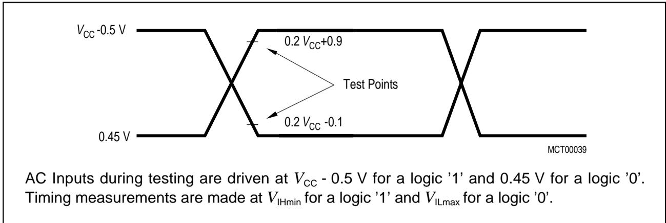
**AC Testing: Input, Output Waveforms**
