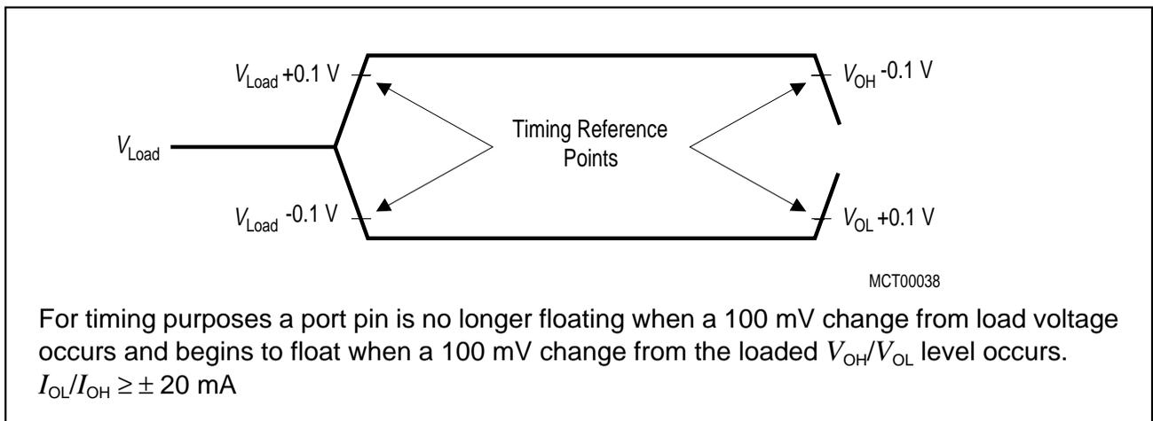
**AC Testing : Float Waveforms**
