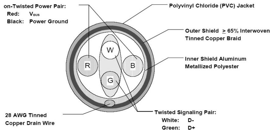
For USB3.0 cabling it is required to use only HiSpeed USB cable, specified in USB3.0 standard:
