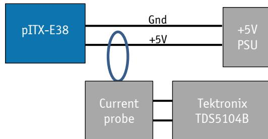
Note that power consumption of the Display and HDD are not included.
