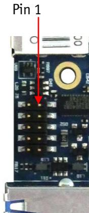
Note1, LED output has integrated 220 ohm.
