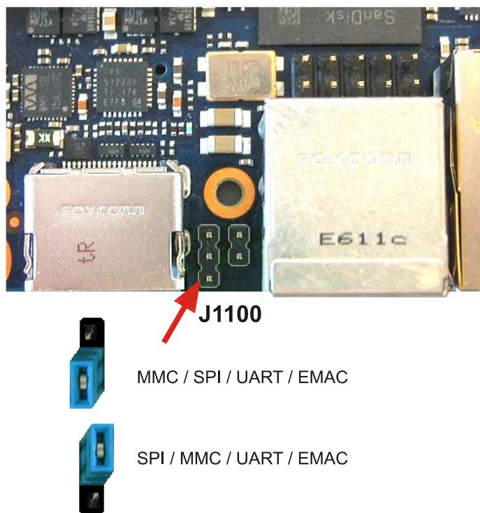
If you use the boot order 'MMC/SPI/UART/EMAC' you can bypass the Kontron bootloader in the SPI flash. This circumstance gives more flexibility for own solutions.
