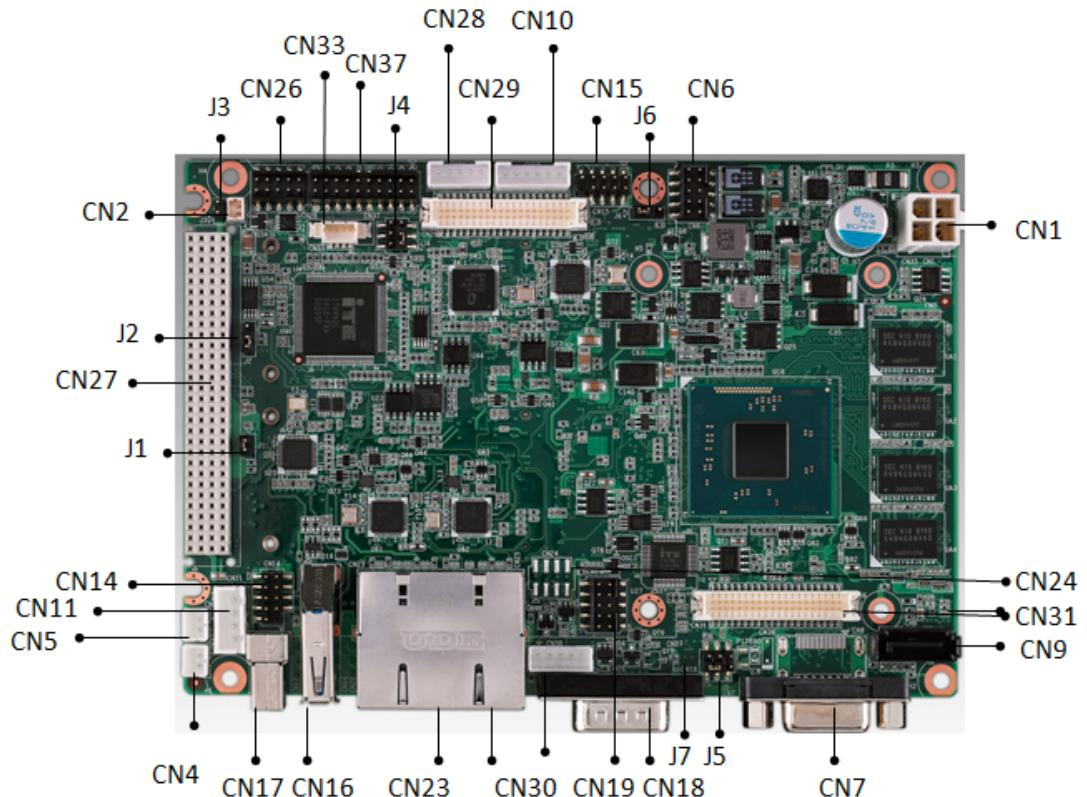
**Figure 2.1 PCM-9365 Connector Locations (Top Side)**
