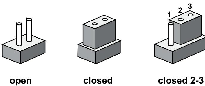
A pair of needle-nose pliers may be helpful when working with jumpers. If you have any doubts about the best hardware configuration for your application, contact your local distributor or sales representative before you make any changes. Generally, you simply need a standard cable to make most connections.
