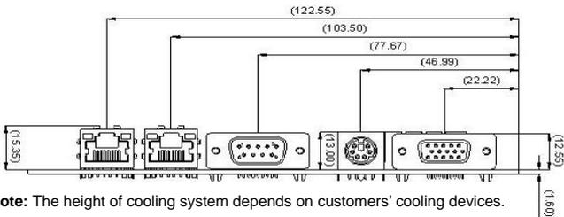
**Note:** The height of cooling system depends on customers' cooling devices.
