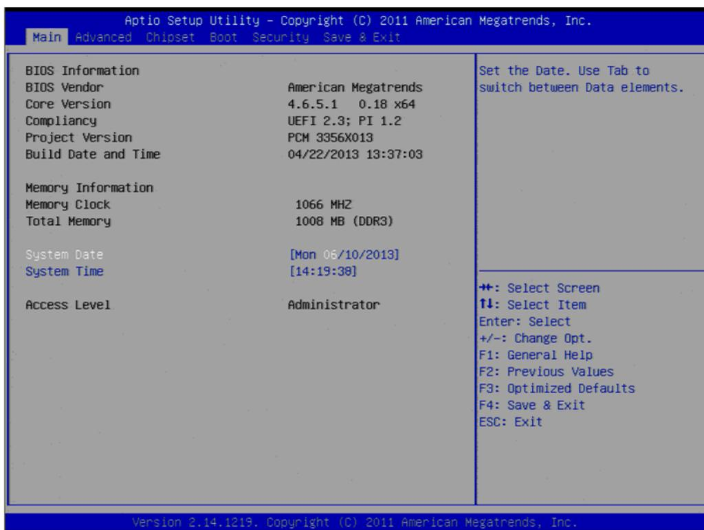
The main BIOS setup screen has two main frames. The left frame displays all the options that can be configured. Grayed-out options cannot be configured; options in blue can. The right frame displays the key legend.
