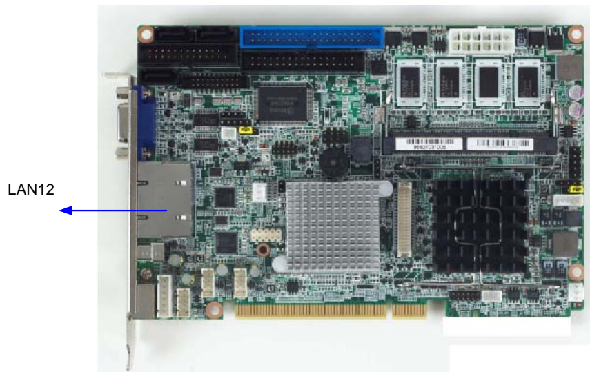
Figure 2.11 Dual Giga LAN RJ45 connector (LAN12)
