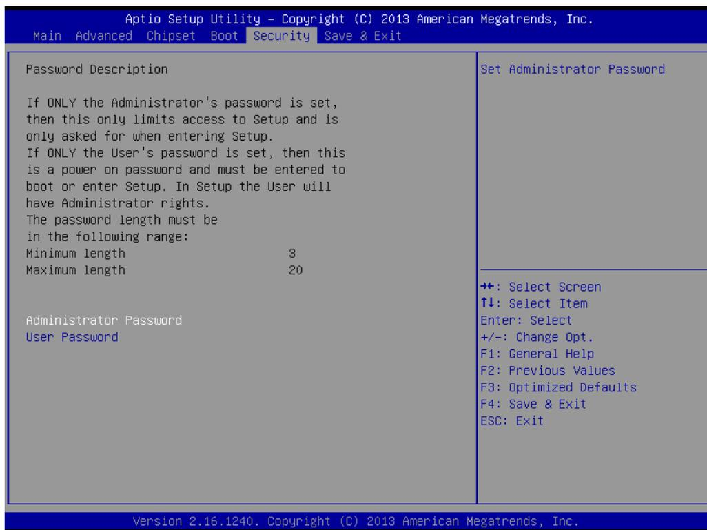
Select the Security tab from the main BIOS Setup Utility menu. All security setup options, such as password and virus protection, can be accessed from this menu. To access the submenu of any item, select the item and press <Enter>.
