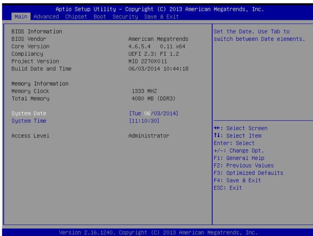
The Main BIOS setup page comprises two main frames. All configurable options are displayed in the left frame. Grayed-out options cannot be configured, whereas the options presented in blue can be configured. The key legend is displayed in the right frame.
