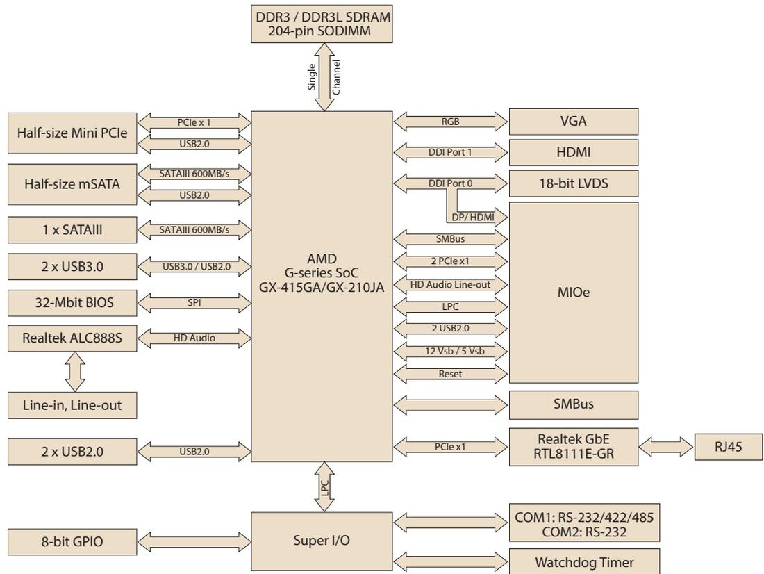
Figure 1.1 Block diagram
