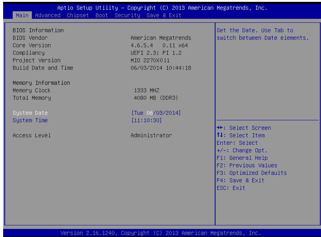
AMI's BIOS ROM has a built-in setup program that allows users to modify the basic system configuration. This information is then stored in flash ROM to ensure that the setup information is retained even when the system is powered off.
