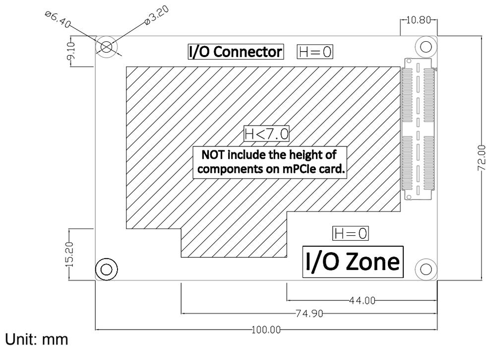
**Figure 2.10 MI/O module height constraints**
