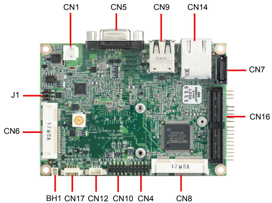
Figure 2.2 Jumper and connector layout (Bottom side)
