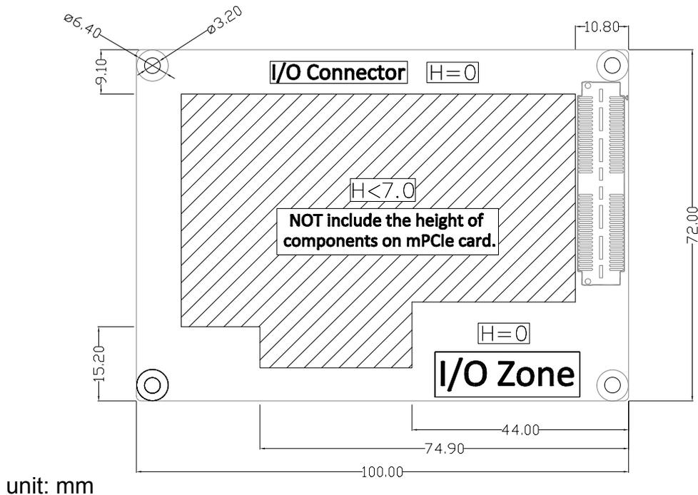
**Figure 2.11 MI/O Module height constraint**
