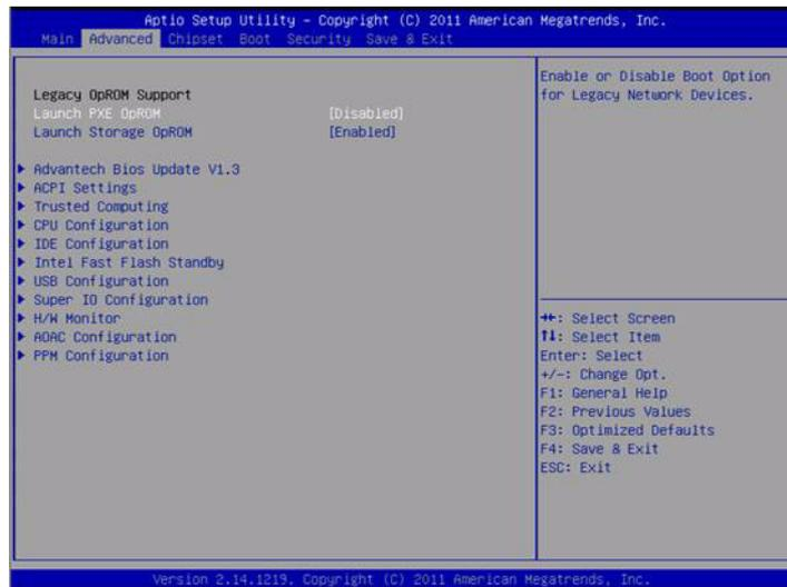
Figure 3.3 Advanced BIOS features setup screen
