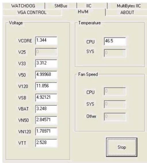
When the Monitor application is executed by clicking the button, hardware monitoring data values will be displayed. If certain data values are not supported by the platform, the correspondent data field will be grayed-out with a value of 0.
