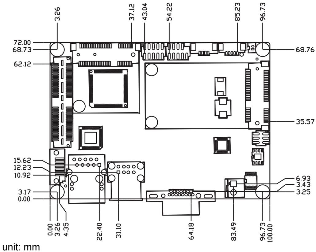
Figure 2.4 Board dimension layout (Bottom side)
