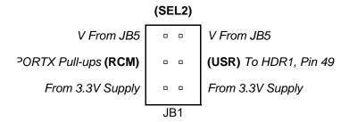
JB1 controls the pull-up voltage of the High Drive Output lines and determines what voltage is present on pin 49 of HDR1. One side of the jumper (USR) controls pin 49 and the other side (RCM) controls the pull-up voltage of Port X. Leaving the USR shunt off leaves pin 49 open and leaving the RCM shunt off sets the High Drive Outputs to no pull-up voltage (open collector). The voltage at the SEL2 pins is defined by JB5.
