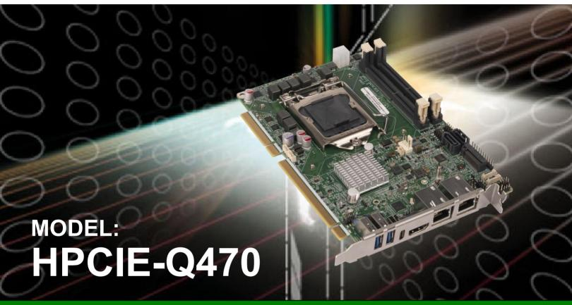
Half-Size PICMG 1.3 CPU Card Supports LGA1200 10<sup>th</sup> Gen Intel® Core™ i9/i7/i5/i3 /Pentium® /Celeron® CPU with Intel® Q470/Q470E, DDR4 SO-DIMM, HDMI, USB-C, Dual Intel® 2.5GbE, USB 3.2, SATA 6Gb/s, M.2, HD Audio, Intel® AMT and RoHS
