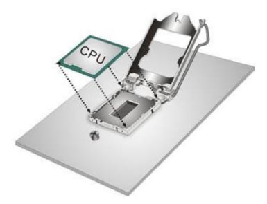
Figure 4-3: Insert the Socket LGA1200 CPU
