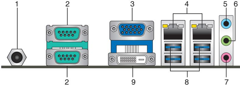
1. **DC power port.** This port connects to a DC power adapter.
