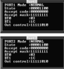
The status fields show information including the Mode (Normal or Reset), Acceptance Code, Acceptance Mask, BTR0, BTR1, Output Control Register, and Status Register. The normal value of the Status Register is:
