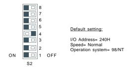
S2 (switch 1 ~ switch 6): COM Port base I/O address setting
