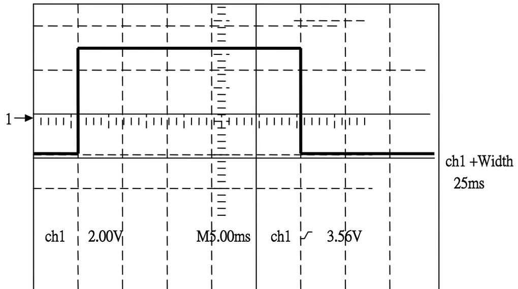
Figure 1. GPS Receiver Time Mark Pulse Waveform.
