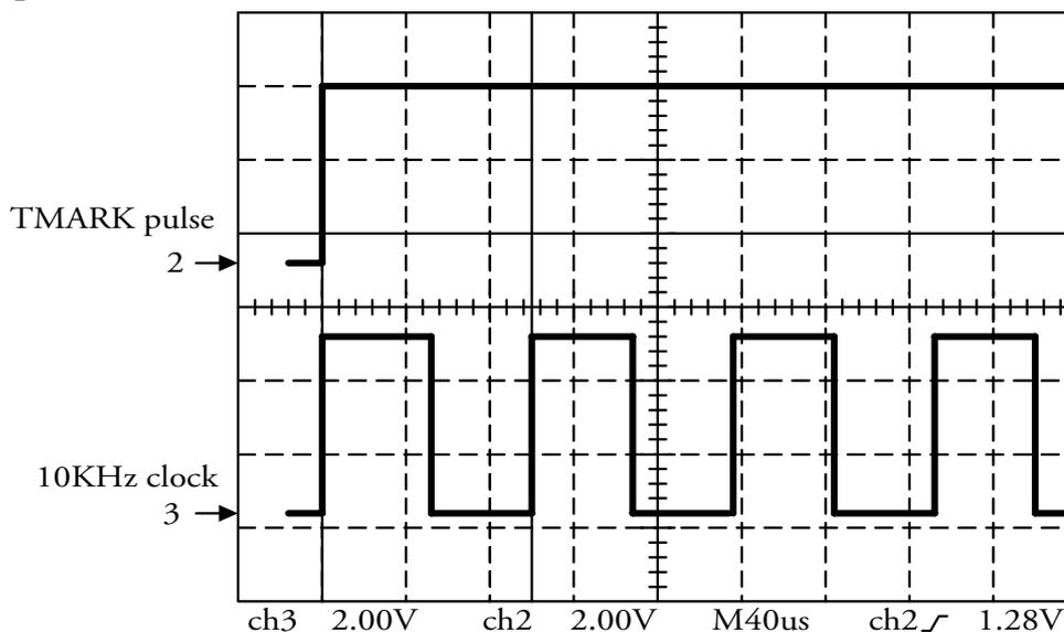
Figure 2. 10KHz Clock/UTC TMARK Pulse Relationship
