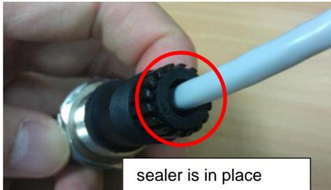
Step 8: Press the cable hard inward and lock the plastic rear nut tightly at the same time.
