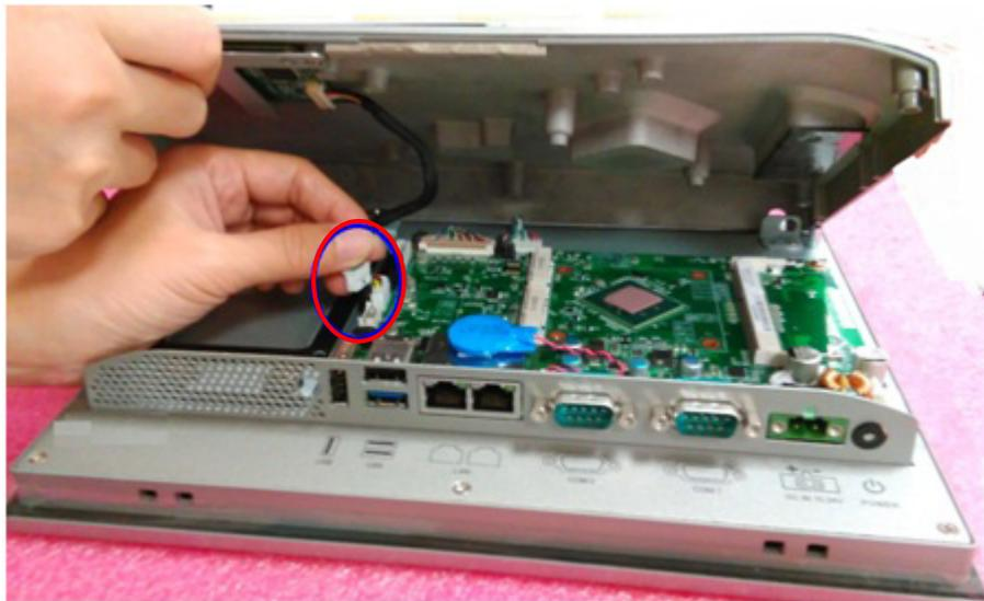
**Figure 2.5 Remove cable from Mainboard**
