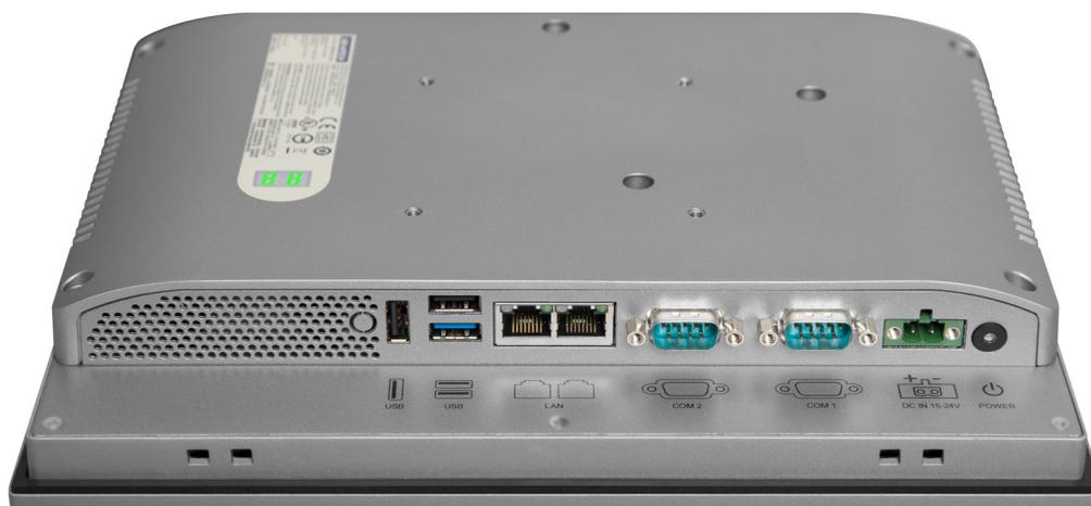
Figure 1.3 Bottom side of PPC-31x0S
