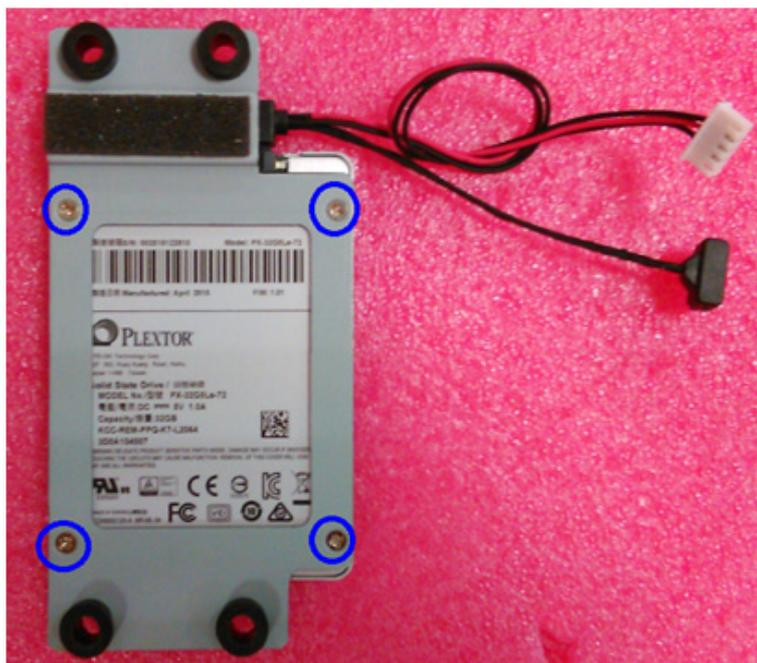
Figure 2.11 Secure SATA HDD with screws
