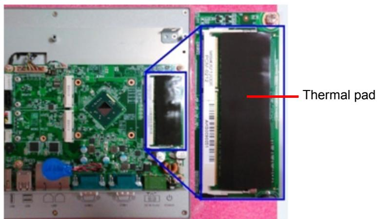
Figure 2.7 Attach thermal pad on memory
