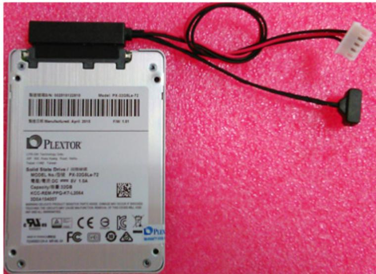
**Figure 2.10 Connection of cable and SATA HDD**
