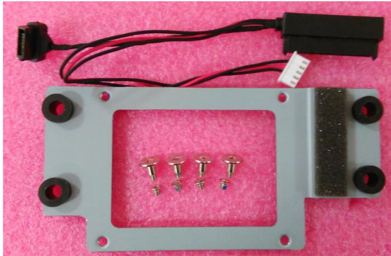
**Figure 2.9 HDD Module**
