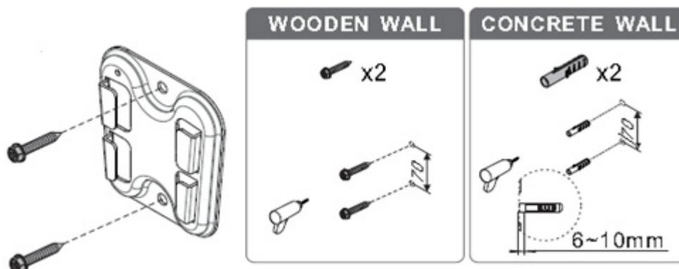
**Figure 2.20 Mounting the Bracket on the Wall**
