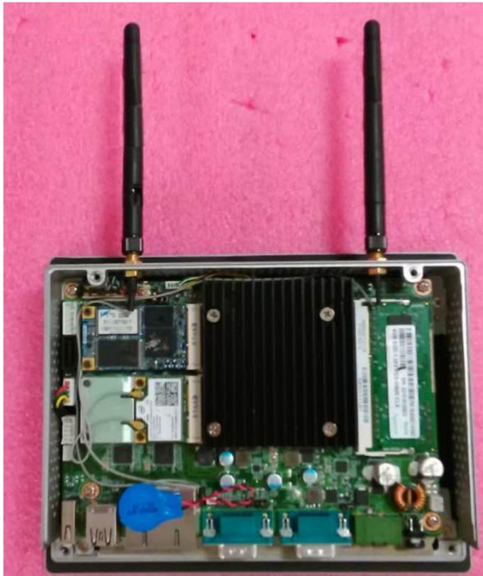
**Figure 2.19 Antenna Cables of Half-size Mini PCIe LAN Module**
