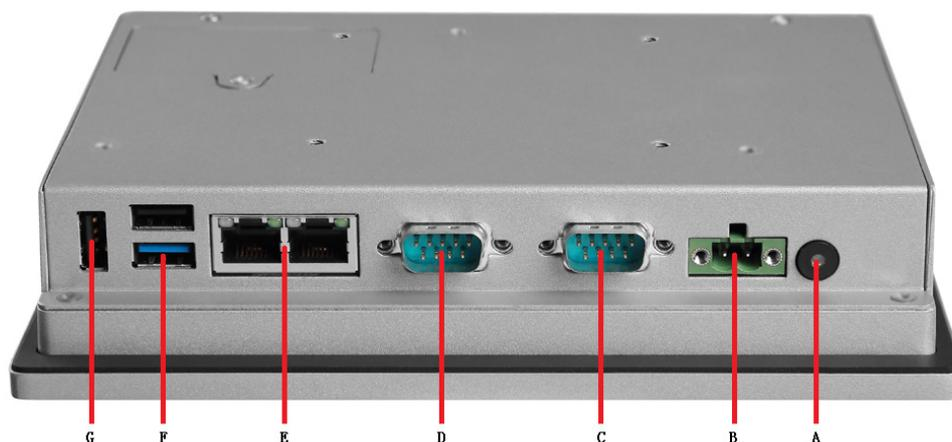
**Figure 2.3 I/O Connectors**
