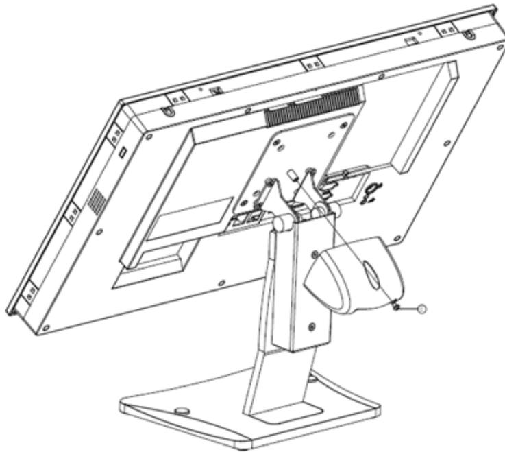
**Figure 2.33 Securing the Hinge Cover**
