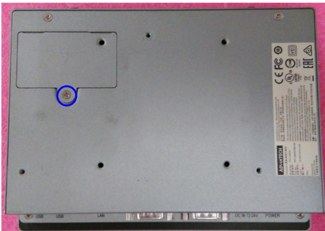
Figure 2.11 Removing the mSATA Door
