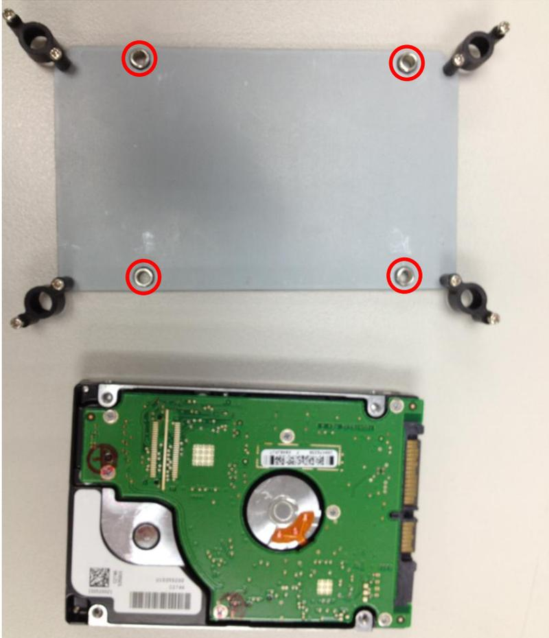
Step 4: Fasten the screws of the hard disk bracket onto the AHP-2173
