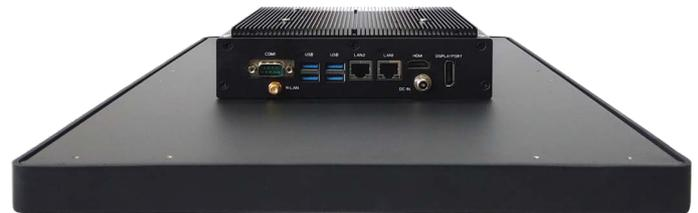
Capacitive PC series stands out among competition with its fanless silent operation, IP65 front panel design, high reliability and fine craftwork.
