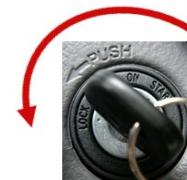
2. The system will shut down 5 minutes later after turning off the vehicle.
