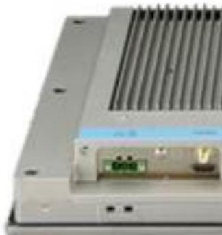
Figure 2.3 Power Receptor
