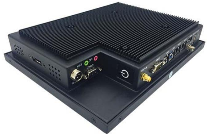
Resistive Touch PC series stands out among competition with its fanless silent operation and robust aluminum housing with stable VESA 100 fixation bolts.
