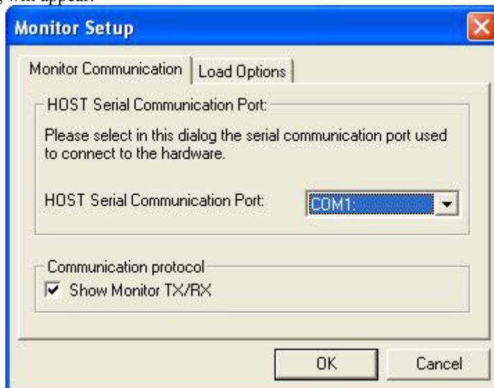
From this dialog you can select the correct serial port if COM1 is not available on your computer. Press OK and if everything is properly configured, you will see the debugger erase the memory and download the program while displaying a progress bar similar to the one shown below:
