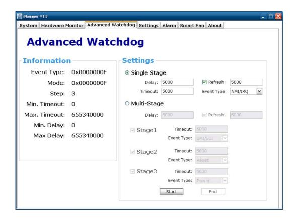
Single stage: In this stage, you can set delay time, refresh time, timeout in milliseconds and event type.
