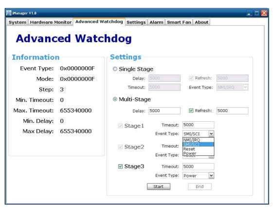
Multi-stage: The multi stage watchdog allows up to 3 actions in each stage; one can set a different timeout in milliseconds based on event type.
