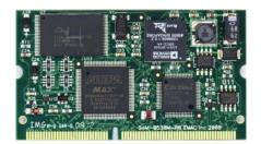
This document describes EMAC's SoM-536EM (SBC) module. The SoM-536EM is a System on Module, designed to be compatible with EMAC's 144-pin SODIMM form factor standard. This module is built around the Analog Devices ADSP-BF536 microcontroller, which provides several of its key features.
