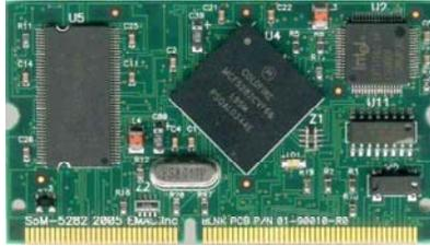
This document describes EMAC's SoM-5282EM (SBC) module. The SoM-5282EM is a system on module, designed to be backwards compatible with EMAC's SoM-400EM, but taking advantage of the more powerful MCF5282 processor.
