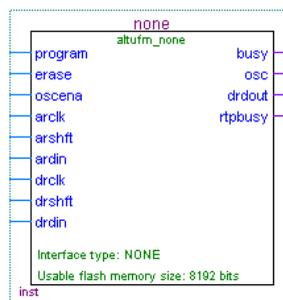
[Figure 10–15](#) shows page 3 of the `altufm` MegaWizard Plug-In Manager, selecting **none** for the interface protocol. By selecting **none**, all the other options are grayed out or unavailable to you. However, you still can specify the initial content of the UFM block in page 4 of the `altufm` MegaWizard Plug-In Manager as discussed in [“Creating Memory Content File”](#) on page 10–24.
