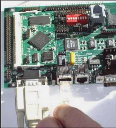
A network connection may be established by connecting the carriers Ethernet jack to a standard 10/100 base-T network.
