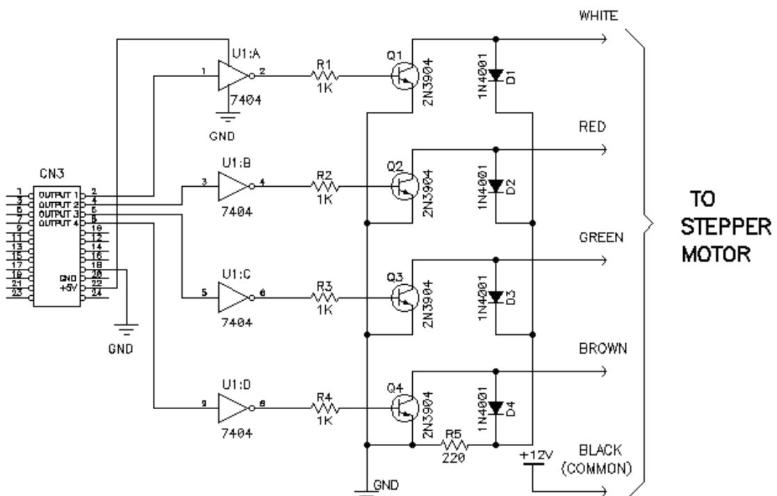
PRIMER is reset. The interface is connected to the low nibble (4 bits) of the PRIMER output port. The driver circuit should be built on a breadboard following the schematic. Once built, a small piece of solid wire should be tightly wrapped around the shaft of the stepper motor to serve as a pointing device.
