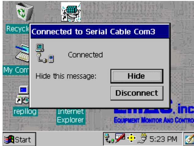
Since Windows CE does not support Partnerships. Active Sync will require a selection of no to Partnerships. At this point you can explore the file structure of the remote device. This type of connection is supported via Embedded Tools (see figure on next page).
