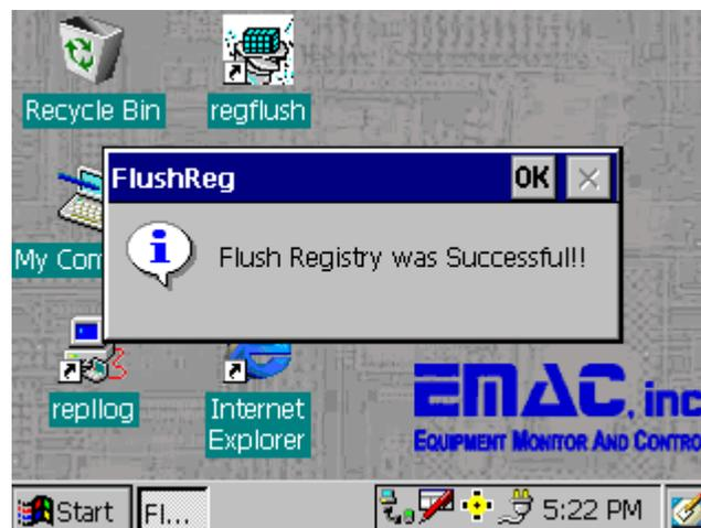
Since Windows CE saves its Registry Entries in volatile RAM, when the system is rebooted the updates are lost. The PPC-E5 Windows CE build contains a driver to write the Registry to the DiskOnChip, resulting in a non-volatile or Persistent Registry. The FlushReg application, that is provided, makes an API call to flush the registry to the DiskOnChip. The sample code below shows an example of API calls in Visual BASIC and Visual C++.
