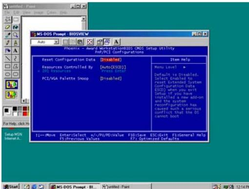
Figure 4.7: PnP/PCI Configurations
