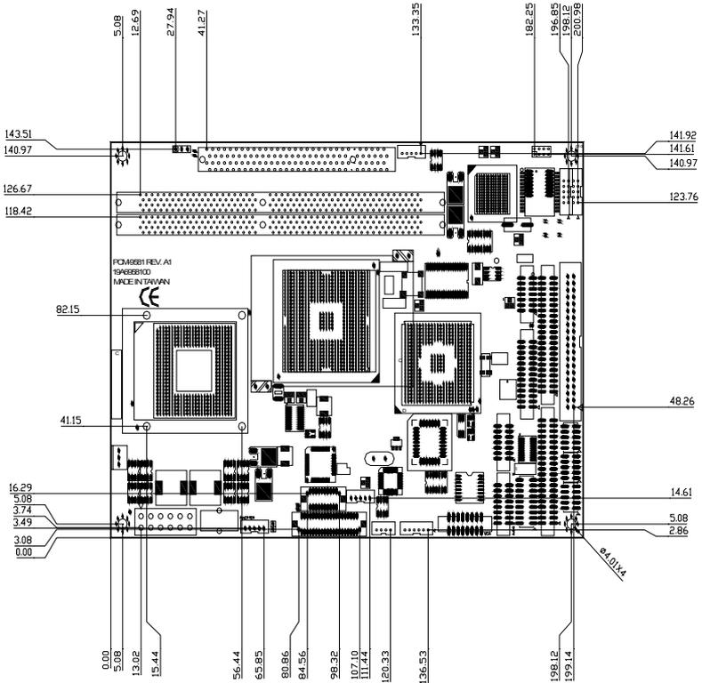
Figure E.1: PCM-9581 Mechanical Drawing (component side)
