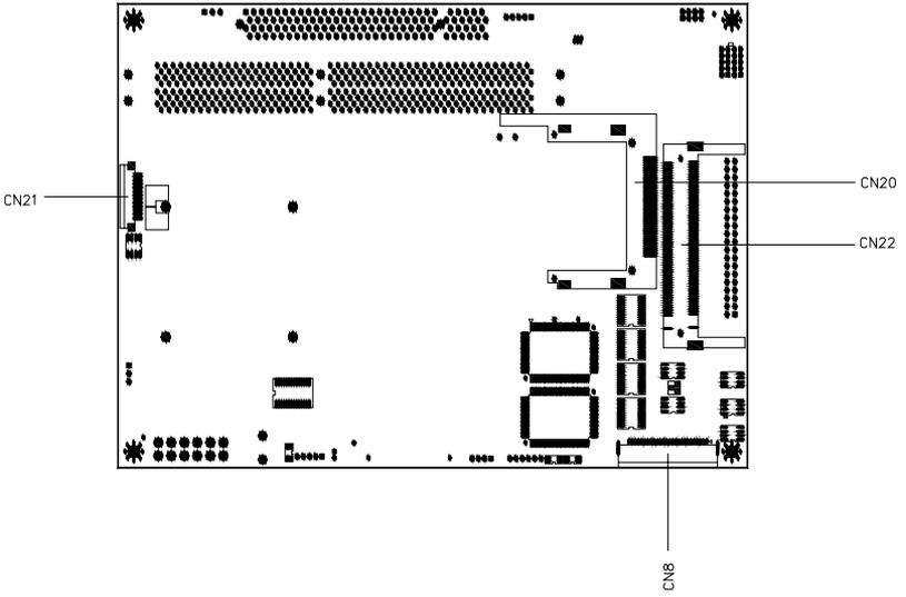
*Figure 2.2: Jumper & Connector (solder side)*
