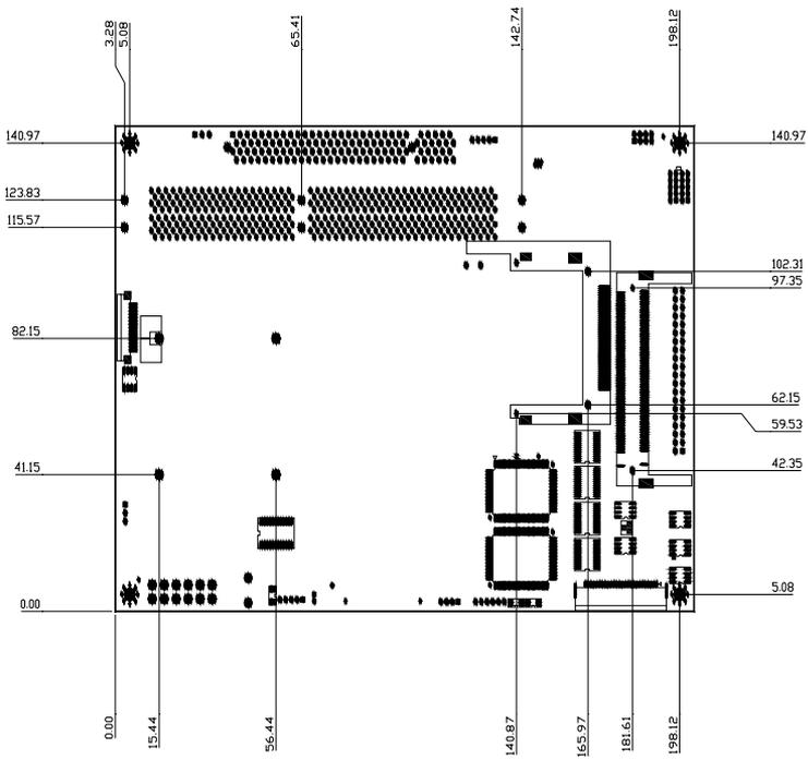
*Figure E.2: PCM-9581 Mechanical Drawing (solder side)*
