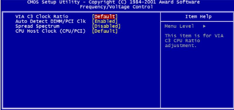
*Figure 4.9: Frequency/Voltage Control*
