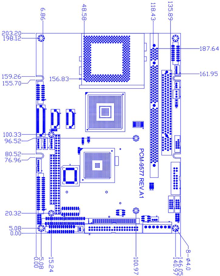
*Figure 1.1: Board layout: dimensions*
