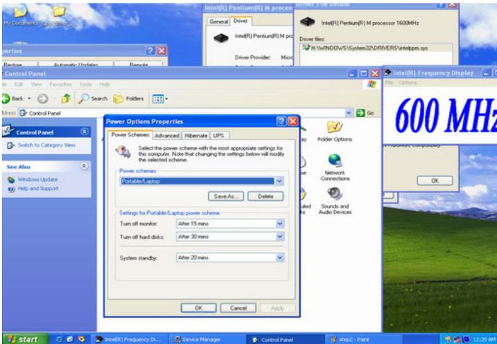
Step 3. Discover the different CPU freq. by using FrequencyDisplay utility
