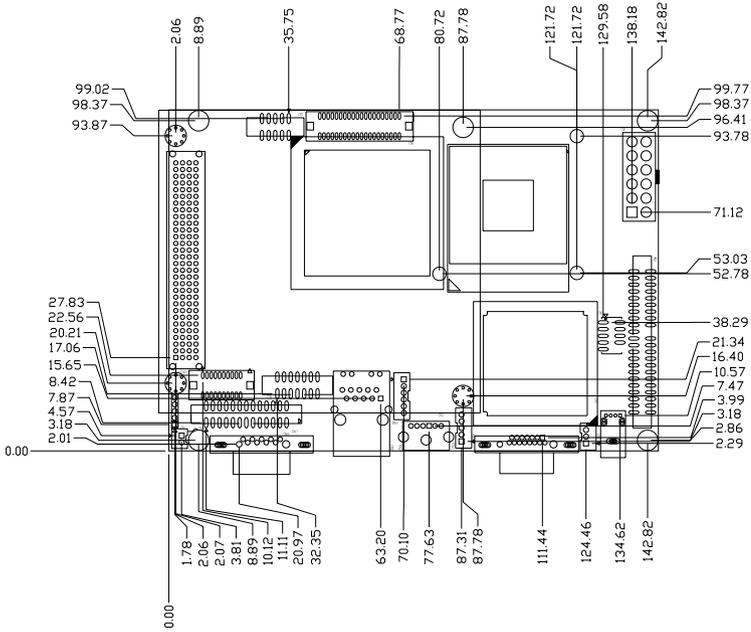
**Figure F.1: PCM-9381 Mech Drawing(Component)**
