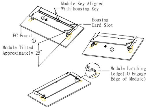
The procedures for installing SODIMMs are described below. Please follow these steps carefully. You can install SDRAM memory modules using 200-pin SODIMMs (Small Outline Dual In-line Memory Modules).
